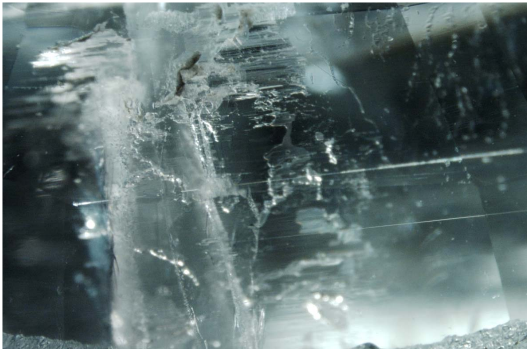
Figure 3: Partially healed fissures in one of the tourmaline selected for diffusion experiments.
