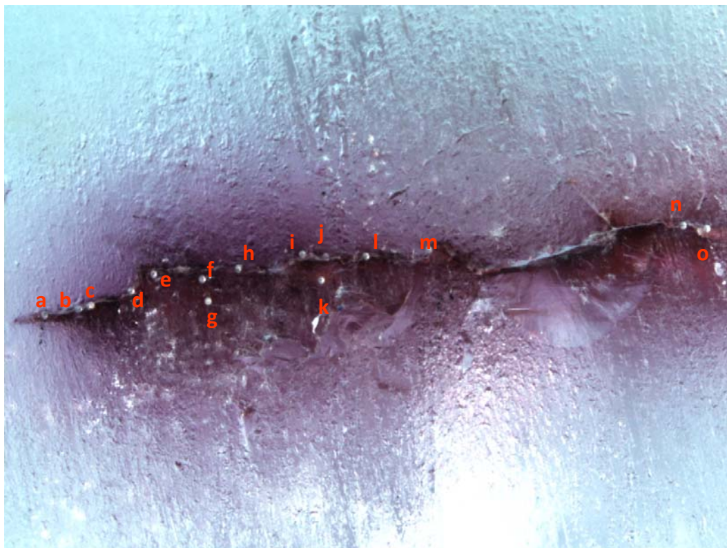
Figure 17 Photomicrograph of the spots analyzed by using LA-ICP-MS after the stone had been ground down 0.5 cm. Each spot was analyzed at the ground down surface (first number in the following pairs for each spot) and 2 \mu m below the surface (second number in the following pairs for each spot).
