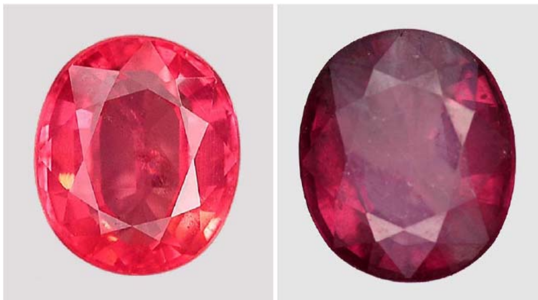
Figure 3: A 1.17ct spinel from Tanzania before heating (left) and after heating at 1400°C, in O 2 , for 5 hrs (right).
