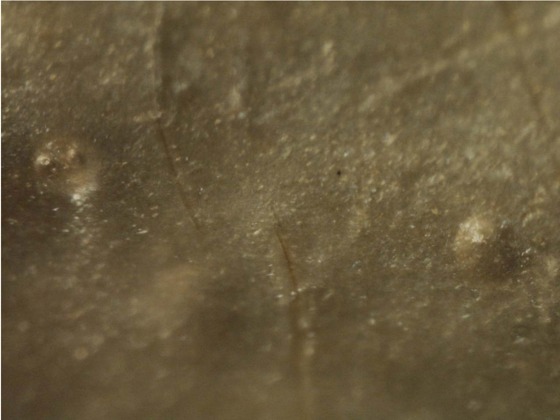
Figure 11: Bubbles visible in the coating used to conceal the opening into the pearl through which the fillers were inserted. Magnified 85x.
